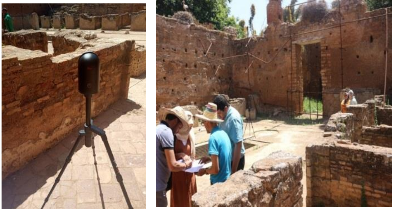
Figure 5. Laser data setting and capturing using Leica scan (Author's figure).
