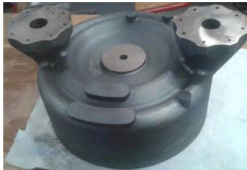
Figure 8. Vulcain 2 jet engine injector, manufactured via usage of SLM technology (Soller et al., 2016).
